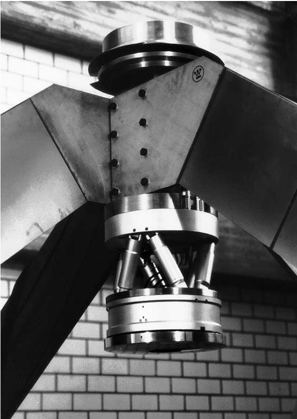
Fig. I.4: The new secondary mirror unit of the UKIRT with a dummy mirror in the workshop at the MPIA.
