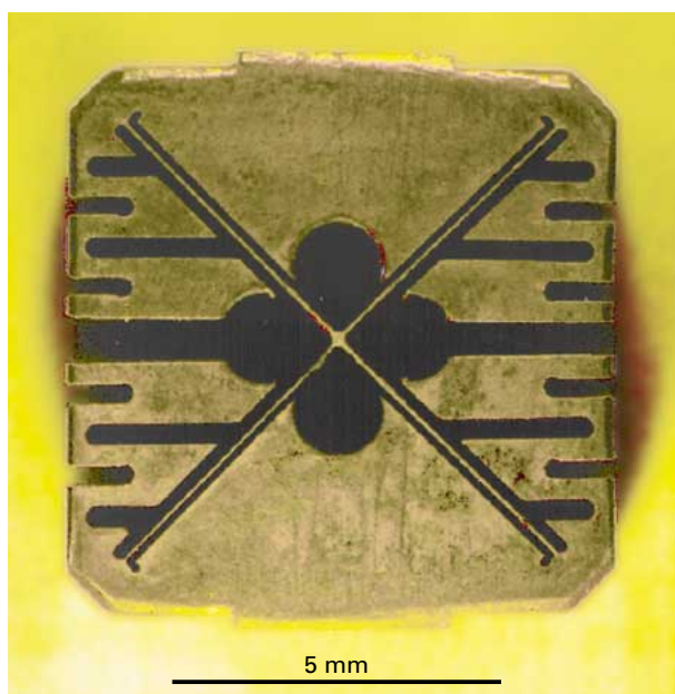
Fig. III.9: Prototype of a cross spring joint on which the chopper axle is mounted.
